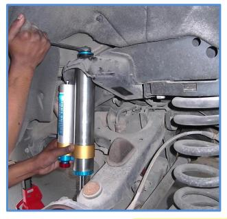
**Important Note:** The rubber bushings on your King shocks are different from each other. Make sure the taller bushing is on the bottom next to the body of the shock as shown. The silver washer between the rubber bushings represents the material thickness of the upper shock mount. It's important to tighten the nut only until the rubber bushings start to compress. There should be approximately 1/8" - 3/16" of the mounting pin protruding above the nut. **\*Do not over-tighten the nut.**
