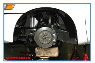
4. Before installing the reservoir bracket, make sure to place the upper hose clamp into position. Then proceed to bolt reservoir bracket into place. The nut for the bracket will go on the back side. When tightening, the reservoir will be almost vertical, it is self-aligning. Lower jack and remove.
