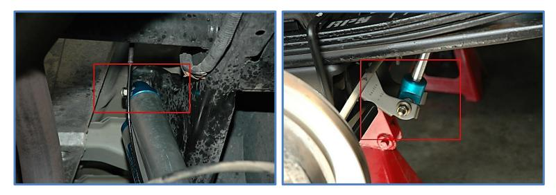
Driver-side (Left) reservoir should face towards the rear of the vehicle and the passenger-side (Right) reservoir should face the front of the vehicle. Make sure longer spacer is towards the frame to space the shock away from frame.
