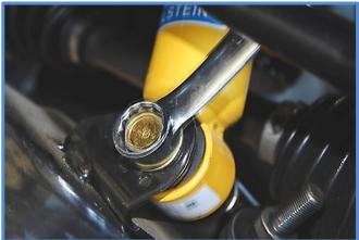
4. To gain more clearance to remove the old shock and to reinstall the new King Coilover shock you must unbolt the ABS bracket using a 12mm wrench or socket. Unbolt ABS bracket and
