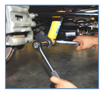
2. You can then remove the upper shock mount nut using a 17mm socket or wrench.
