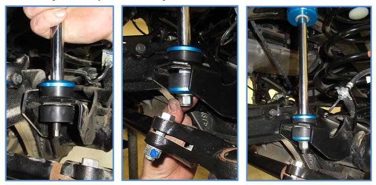
4. Attach the reservoir clamps to the reservoir bracket using the supplied hardware. Place the clamp on bracket as shown and install the 2 BHCS (CB2420). Be sure to use high strength thread lock to prevent clamp from vibrating loose.
