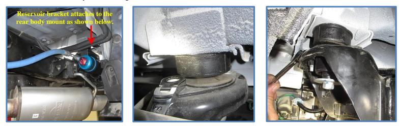
6. Attach the reservoir clamps to the reservoir bracket using the supplied hardware. Place the clamp on the bracket as shown below and install the provided 1/4 X 1/2" BHCS (CB2420). Use high strength thread lock on these screws to ensure the clamps stay secure.
