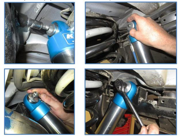
4. Place the spacer on the lower mounting stud followed by the rod end, then place the other spacer on the mounting stud and install the factory washer and nut. Tighten all hardware to factory specs.
