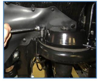
3. Unbolt and remove the factory bump stop.
