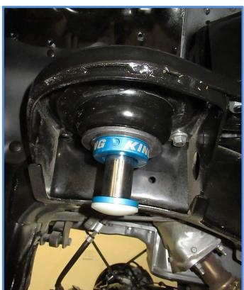
10. Cycling suspension and adjusting bump stops – Now that the bump stops are installed you will need to adjust the position so the bump stop is setup properly for your vehicle. With the coil springs removed and the shocks installed, jack the axle up until the shocks are bottomed out (Fully Compressed). Now adjust the bump stop so that it bottoms out just before the shock does.
