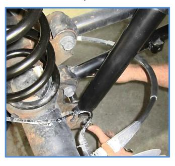
3. Using the supplied custom wrench, remove the upper mounting bolts and remove shocks.
