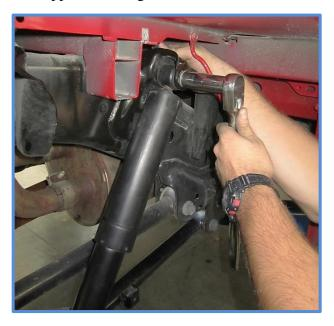
4. Install King Shocks with the reservoirs up and the shaft mounted to the axle. Also make sure the longer bearing spacers are pointed inward to properly offset the shocks. Reinstall the factory bolts and tighten to factory specs, Reinstall the plastic wheel well piece in the reverse order it was removed.
