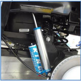
4. On the passenger side (Right side) you may need to pull some slack from the parking brake cable in order to fit the shock. Grab the metal sleeve with pliers and twist the sleeve while pulling the cable through the sleeve. You should only need ½" – ¾" or so, check the fit and adjust accordingly.
