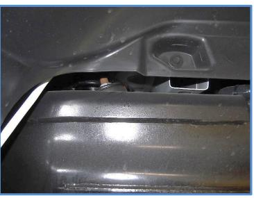
2. Remove the nut and bolt from the lower mount using a 21mm socket/wrench and remove shock.
