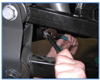
Important Note: The rubber bushings on your King shocks are different from each other. Make sure the taller bushing is on the bottom next to the body of the shock as shown. The silver washer between the rubber bushings represents the material thickness of the upper shock mount. It's important to tighten the nut only until the rubber bushings start to compress. There should be approximately 1/8" – 3/16" of the mounting pin protruding above the nut.
