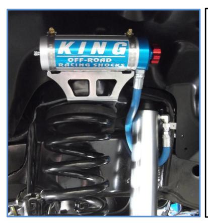
Important Note: The rubber bushings on your King shocks are different from each other. Make sure the taller bushing is on the bottom next to the body of the shock as shown. The silver washer between the rubber bushings represents the material thickness of the upper shock mount. It's important to tighten the nut only until the rubber bushings start to compress. There should be approximately 1/8" – 3/16" of the mounting pin protruding above the nut.
