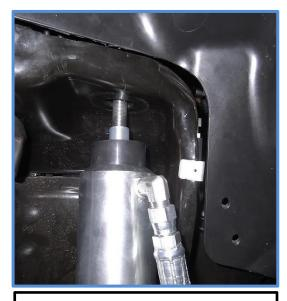
This is the view of the driver's side (left side) make sure the shock is installed so the fitting is angled back towards the rear of the vehicle and the shock is rotated so the fitting is as far back as possible without touching the body. Also notice that the large bushing is on the bottom.
