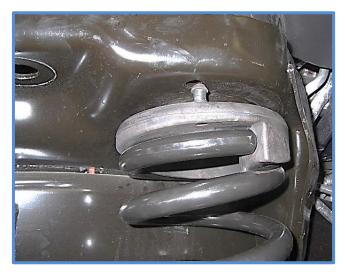
6. Place the reservoir brackets in position on the rubber isolators so the hole for the locating pin lines up. Jack the axle up slowly while checking both sides to make sure the coil is seating properly. Make adjustments as necessary and continue jacking the axle up until the coil begins to compress.
