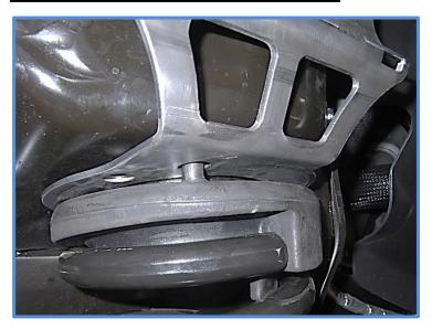
4. Now with both front shocks removed you can lower the front axle until the springs are loose. You will be mounting the reservoir bracket between the rubber spring isolator and the upper spring mount.
