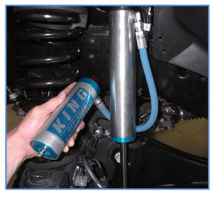
10. With the hose properly routed and the reservoir installed you can install and tighten the original lower shock bolt and tighten the upper nut.
