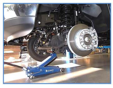
2. Remove the front shocks - Remove the nut from the upper shock mount using an 18mm wrench.
