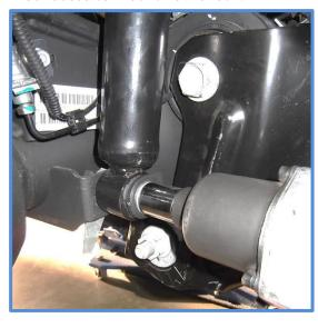
5. Lower the axle until you can slide the reservoir bracket between the rubber spring isolator and the upper spring mount.
