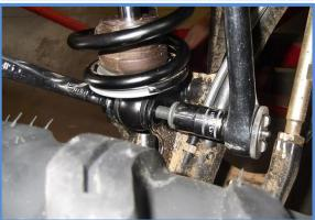
2. Install King Shocks using the factory hardware. Shocks are side specific. Be sure to mount the shocks properly with the reservoirs facing back as shown.
