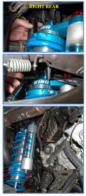
Double check your install, make sure the shocks are mounted properly and all hardware is tight. Recheck the hardware after 50 miles and periodically after that as part of routine maintenance.
