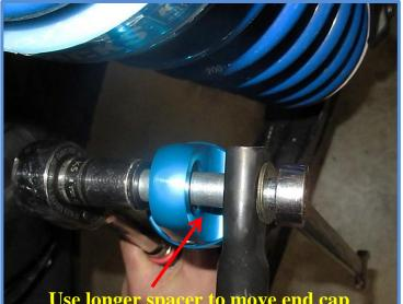
Use longer spacer to move end cap away from sway bar to avoid sway bar hitting end cap at full compression.
