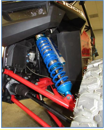
Double check your install, make sure the shocks are mounted properly and all hardware is tight. Recheck the hardware after 50 miles and periodically after that as part of routine maintenance.
