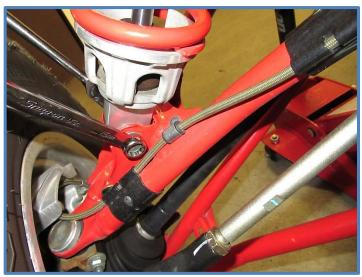
3. Remove the upper mounting bolt using a 15mm wrench and socket then remove shock from vehicle.
