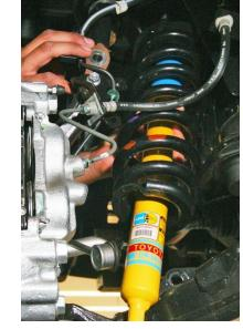
(4) Remove the bolt holding the ABS line from the spindle. While holding the ABS line out of the way, remove the lower shock bolt and pull the factory shock out from the bottom.
