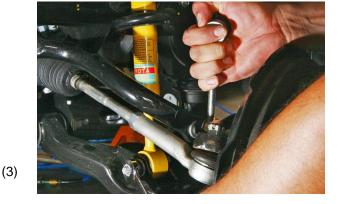
(3) Remove the nuts from the upper and lower shock mounts but leave the bottom bolt in for now.
