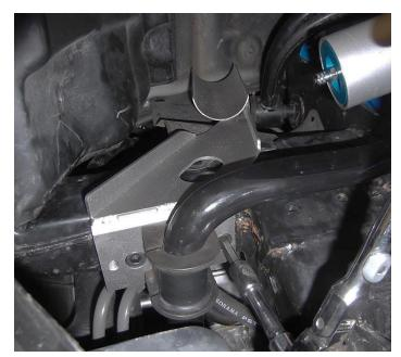
(6) Re-attach the sway bar end link. Bolt the remote reservoir mount into the sway bar mount holes with the supplied M10 x 40mm allen head bolts.
