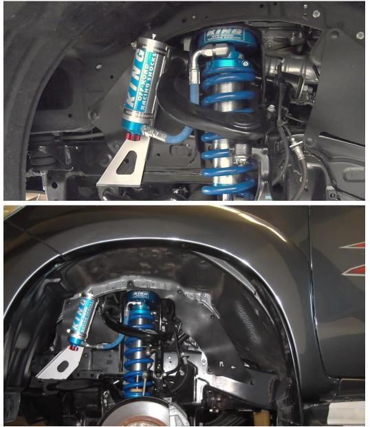
**DOUBLE CHECK ALL HARDWARE:** Make sure everything is installed correctly and all hardware is tight before reinstalling tires. Install tires, remove jack stands and lower vehicle to the ground. Recheck all hardware and lug nuts after 100 miles and periodically after that as part of routine maintenance.
