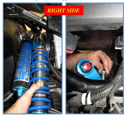
5. Install the factory bolt in the lower mount. Now tighten upper and lower bolts to factory specs.
