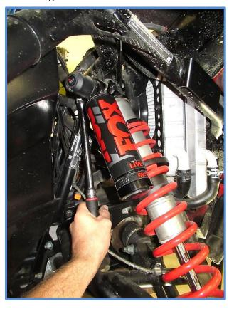
4. Install King Shocks using the factory hardware. Be aware the shocks are side specific. Place the shock in position with the reservoir towards the rear of the vehicle and install the factory bolt in the upper mount first.
