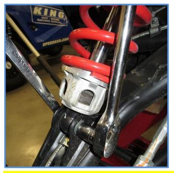
2. Next unplug the wiring connecter at the reservoir and unclip wire from shock. (If Applicable)
