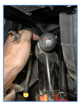
4. Install King Shocks using the factory hardware. Place the shock in position with the reservoir towards the rear of the vehicle and install the factory bolt in the upper mount.
