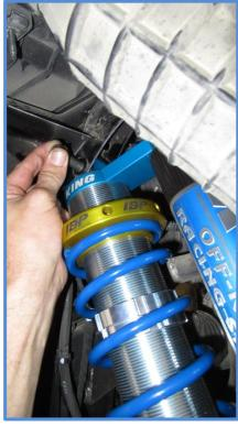
5. Install the factory bolt in the lower mount. Now tighten upper and lower mounting bolts to factory specs.
