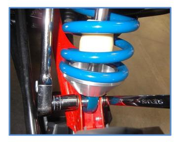
Double check your install, make sure the shocks are mounted properly and all hardware is tight. Recheck the hardware after 50 miles and periodically after that as part of routine maintenance.
