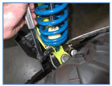
Photo below shows proper shock orientation.
