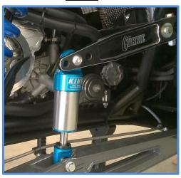
Double check your install, make sure the shocks are mounted properly and all hardware is tight. Recheck the hardware after 50 miles and periodically after that as part of routine maintenance.
