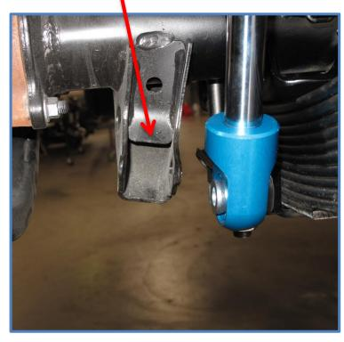
4. Place the reservoir in the reservoir bracket and install the hose clamps through slots in bracket and tighten.
