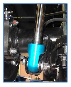
Important Note: The rubber bushings on your King shocks are different from each other. Make sure the taller bushing is on the bottom next to the body of the shock as shown.
