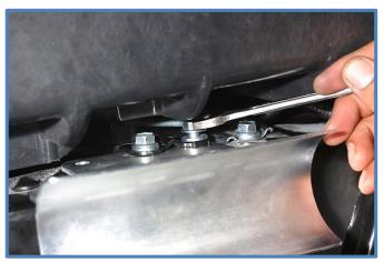
On the opposite side (right) mount the bracket with the provided 8mm bolts (CB3825) and 8mm nuts (CN1801) using the existing holes in the frame.
