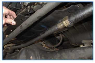
2. Remove the nuts on both ends of the factory steering stabilizer using a 17mm socket/wrench. You may need a ball joint tool or pickle fork to separate the tapered ends from the mounts.
