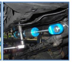
Double check your install, make sure the stabilizer is mounted properly and all hardware is tight. Recheck the hardware after 50 miles and periodically after that as part of routine maintenance.
