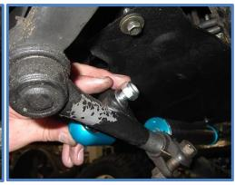
4. Install cylinder end to the factory mount on the opposite side. Insert the tapered spacer into the factory mount. Install the provided 10mm hardware as shown and tighten nut to 50 ft/lbs.
