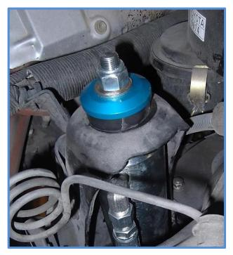
9. The finished install should look like the photo to the right... Make sure everything is installed properly and double check all hardware. Install the tires, remove jack stands and lower the vehicle to the ground. Recheck all hardware and lug nuts after 50 miles or so and periodically after that as part of routine maintenance.
