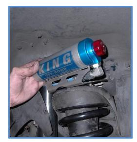
6. Install the provided hose clamps and tighten.
