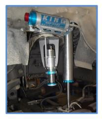
7. Install springs - Unbolt the lower shock mounts, lower the axle enough to install coil springs. Place springs over the bump stop bracket and align with the lower spring perch on axle. Jack axle back up so you can reinstall the lower shock mount hardware. Tighten lower shock mount nuts.
