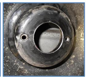
5. Install bump stop brackets – Line up holes in brackets with the nut plate and install the 3/8 x 1" bolts with washer, be sure to use red lock tight. Tighten bolts to 35 ft/lbs.
