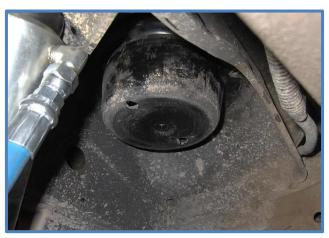
3. Using a 2 ½" hole saw, cut a hole in the center of the bump stop mount using the threaded hole in the center as a guide for the pilot bit.
