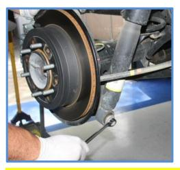
2. Mount the reservoir bracket - Remove the two bolts holding the rubber bump stop to the frame. Place the reservoir bracket between the bump stop and frame and replace the two bolts as shown in the photos below.
