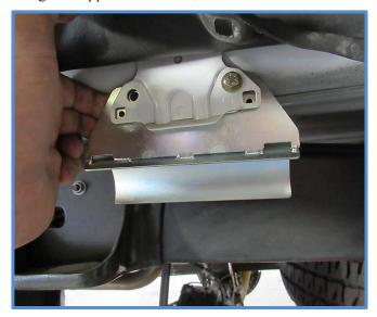
5. Tighten both mounting bolts using a 7/16 wrench and socket. Then let the plastic fender liner down and install the supplied push rivet into the hole.
