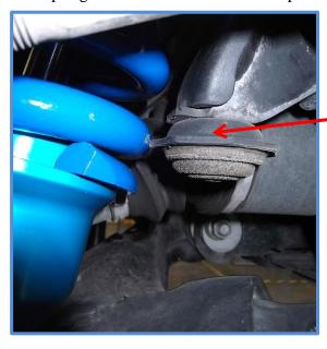
Rotate the bump stop pad or grind any material making contact with the shock at full droop.
