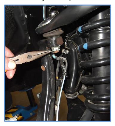
5. Remove upper ball joint nut using a 19mm socket. Separate upper A-arm from spindle.
