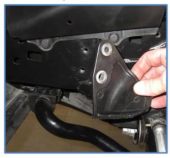
14. Pull the two plastic push pins from the plastic guard and flip up to install reservoir bracket and reservoir.
