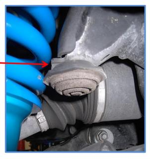
12. Connect upper control arm and tighten to factory specs. Reconnect ABS/brake line brackets.
