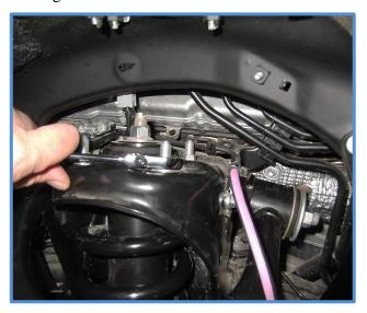
8. Remove the lower mounting bolt using a 22mm wrench and socket. Remove shock from vehicle.
