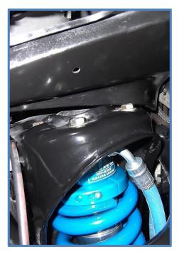
10. Install the factory lower mounting bolt and check clearance at full droop as shown in step 11 on the next page. Make any necessary adjustments, then install factory hardware and tighten to factory specs.
