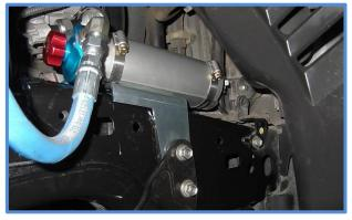
For KDSS Models... You may need to loosen the bracket that supports the hydraulic lines for the KDSS System on the left side of the vehicle. Remove bolt, install reservoir, then reinstall bolt and reposition bracket if necessary and tighten everything once positioned properly.
