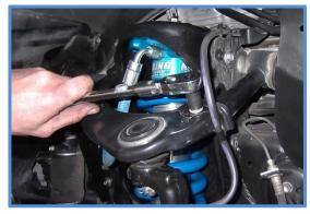
Reconnect the wiring harness bracket at the top of the coil bucket.
