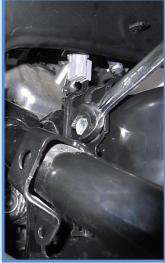
7. Remove the four nuts from the upper mount using a 14mm wrench or socket.
