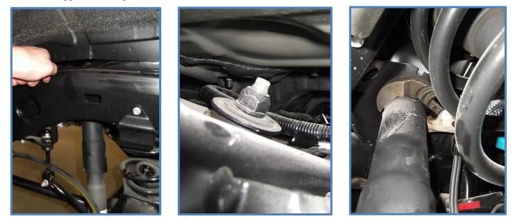
3. <u>Install reservoir brackets</u> – First remove the three bolts holding the bump stop bracket to the frame.
