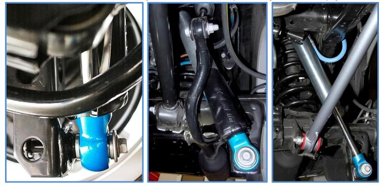
7. Tighten upper nut using a 3/4" wrench.
