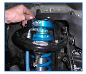
8. Install reservoir in the reservoir bracket using the provided hose clamps. Position the reservoir so it is centered in the cradle with the hose pointing straight back. Adjust accordingly.
