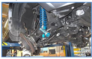
9. Install reservoir brackets using the provided hardware. Thread the 12mm bolt into the cross member, then insert the  $7/16 \ge 3^{3}/4^{\circ}$  bolt through the frame. Install washer, nut and tighten.
