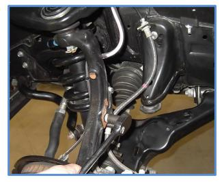
5. Remove upper ball joint nut using a 19mm socket. Separate upper A-arm from spindle.
