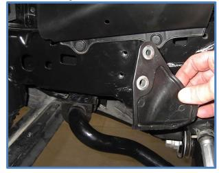
13. Pull the two plastic push pins from the plastic guard and flip up to install reservoir bracket and reservoir.
