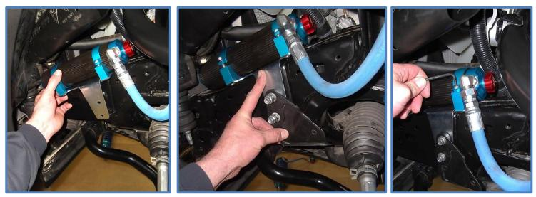
16. The plastic guard can be trimmed to fit around the hose fitting and reinstalled or you can simply remove the guard completely. Photos below show examples of both.
