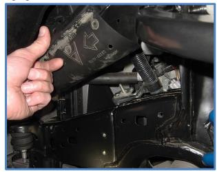
14. Install reservoir clamps to bracket using the provided 1/4 x 1/2" screws (use red locktite). Slide reservoir into bracket.
