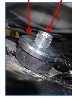
4. Place provided spacer on the lower shock mounting stud. Then place rod end on stud and install the provided 12mm bolt with 7/16 washer. DO NOT reuse the factory bolts.
