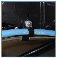
12. Adjust hose: Make sure hose and or fittings are not in contact with frame or body mount. You can rotate the shock and or the reservoir or adjust hose as needed for a clean install. Shocks are built as close as possible to the required hose clocking but some adjustments may be necessary.
