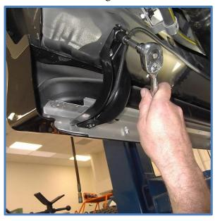
8. Install reservoir brackets behind the side step brackets and reinstall the factory bolts. Reservoir brackets are side specific, see photos below for proper orientation.
