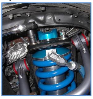
14. Tighten lower factory bolt to 100 ft-lbs. with a 19mm wrench and socket.
