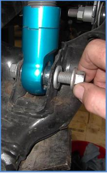
12. Jack up the lower control arm so the upper mounting plate is tight against the upper mount and install the 3/8 HD washers (CW1701) and 3/8 nuts (CN2711).
