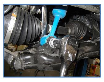
7. Remove the three upper mounting nuts using a 14mm wrench or socket, then remove shocks.
