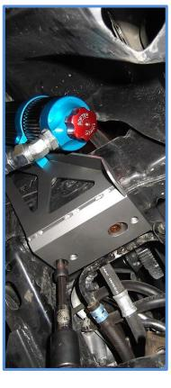
23. Bolt the sway bar to the bottom of the reservoir bracket using the supplied 3/8 X 3/4" bolts (CB4702). Tighten bolts to 35 ft-lbs. Repeat steps 20-23 on opposite side of vehicle. Reinstall skid plate after both sides are done.
