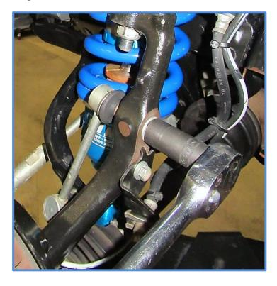
25. Center the reservoir in the clamps and install the 1/4 X 1" SHCS (CB1501). Tighten clamps with a 3/16 Allen wrench.
