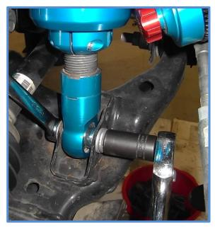
15. Connect the upper control arms using the instructions provided with your UCA kit. Now is a good time to check clearance with the UCA and shock installed, cycle the UCA past the fittings and make sure the UCA does not make contact with hose or fittings. It may be necessary to adjust hose and fittings depending on your set up.
