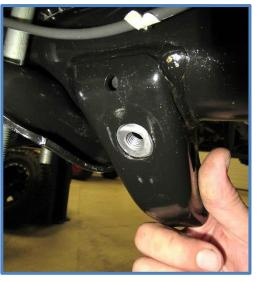
3. Place the shock mount extension over the existing mount and line up the holes in the bracket with the holes on the existing mount. Thread the 1/2 X 1" bolt (CB4704) with washer (CW1702) into the square nut and leave loose for now.
