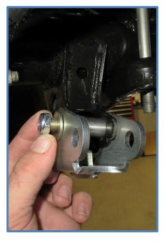
5. Now tighten the  $1/2 \times 1$ " bolt on the back side of the bracket using a 3/4 socket, make sure the bracket pulls in tight to the existing mount.
