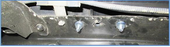
12. Slide the reservoir into the clamps, center the reservoir and install the 1/4 X 1" SHCS (CB1501) and tighten using a 3/16 Allen wrench.
