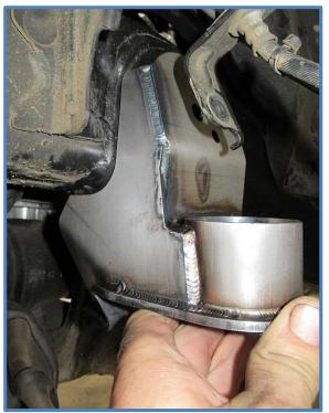
8. Once test fitting is complete, prep the vehicle for welding by removing the paint all the way around the front and sides of the modified factory bracket.
