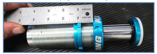
8. Now place the bump stop in the bracket and thread the upper lock ring onto the bumpstop.
