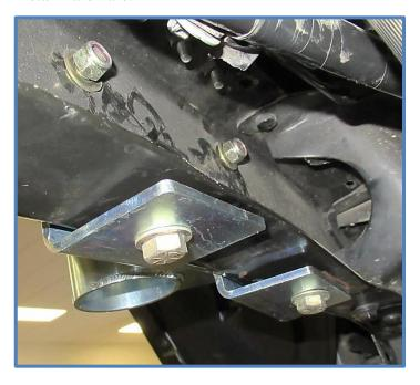
4. Tighten the lower bolts first using a 5/8 wrench and socket, then tighten the upper bolts.
