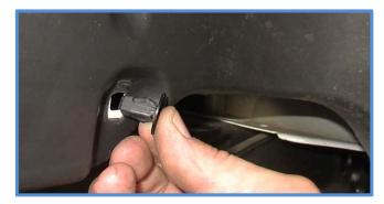
5. Pull fender liner back and install reservoir brackets to the existing holes in the tab hanging down from the bed. Use the supplied 1/4" hardware from the kit. Then let the liner down and insert the supplied push rivet.
