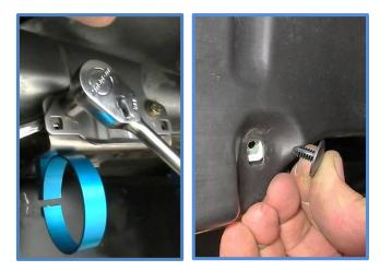
6. Install shock – first remove the nut, steel retainer and upper rubber bushing from the King shock. Feed the reservoir into the clamps as you place the shock up into the upper mount.
