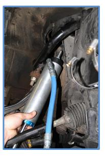
3. Replace the upper bushing, retaining washer, washer and nut. Tighten nut until bushings start to compress.
