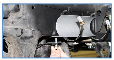
6. The reservoir mounts with hose fitting pointing up. Make sure hose does not interfere with moving suspension parts. Install hose clamps as shown, tighten clamps then tighten remaining bolts.
