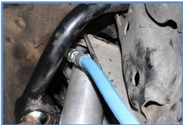
Important Note: The rubber bushings on your King shocks are different from each other. Make sure the taller bushing is on the bottom next to the body of the shock as shown. The silver washer between the rubber bushings represents the material thickness of the upper shock mount. It's important to tighten the nut only until the rubber bushings start to compress. There should be approximately 1/8" of the mounting pin protruding above the nut.
