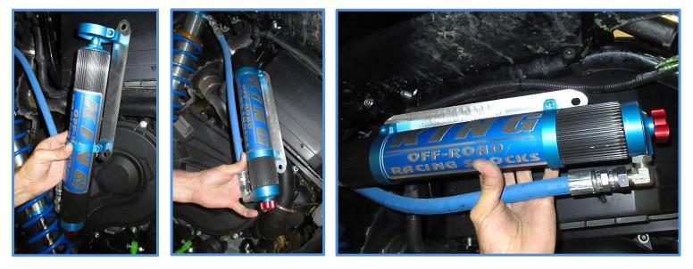
7. Now place the reservoir bracket over the front bolt and between the rear support brackets, line up holes in rear and reinstall the bolt. Install nut on front bolt and tighten to factory specs.
