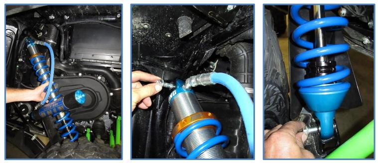
3. Install reservoir brackets – First attach the reservoir clamps to the reservoir bracket using the supplied  $\frac{1}{4} \times \frac{1}{2}$ " BHCS as shown below. Apply locktite to the screws and tighten with a 5/32 hex key.
