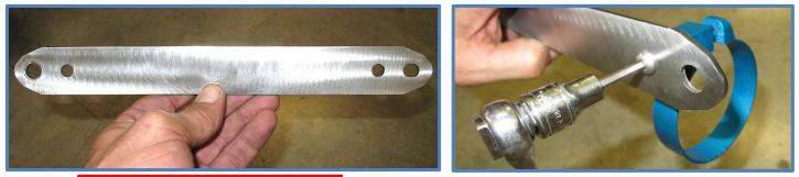
Photos shows left side with large hole in front and the smaller slotted hole to the rear with the clamp hanging down. Right side will be a mirror image of this.
