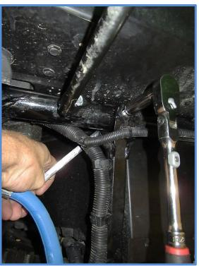
5. Then remove the bolt from rear fender support bracket using a 12mm socket.
