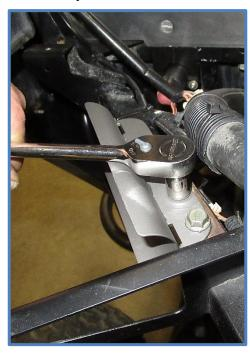
5. Place the reservoir in the bracket as shown. Slide the hose clamps through the slots on either end of the bracket and tighten.
