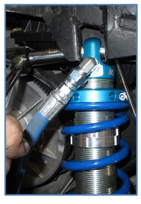
3. Place the rod end in the lower mount, install the factory bolt and tighten to factory specs.
