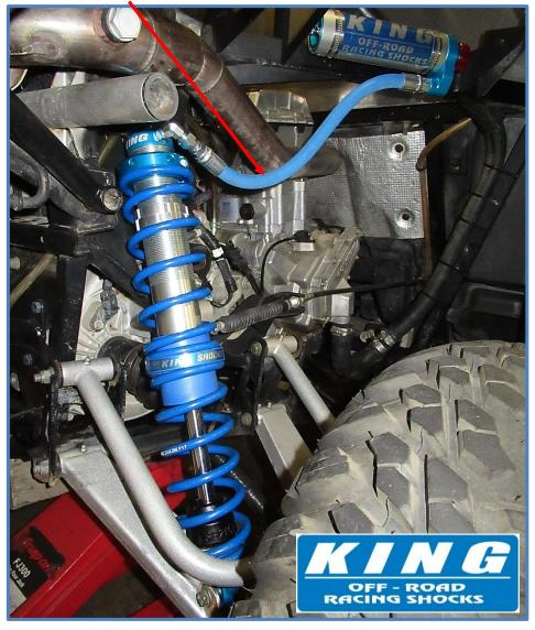
Double check your install, make sure the shocks are mounted properly and all hardware is tight. Recheck the hardware after 50 miles and periodically after that as part of routine maintenance.
