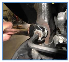
7. Pull the pin from the upper ball joint, loosen nut using a 19mm Socket and separate upper control arm from the steering knuckle.
