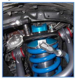
17. Tighten lower factory bolt to 100 ft-lbs. with a 19mm wrench and socket.
