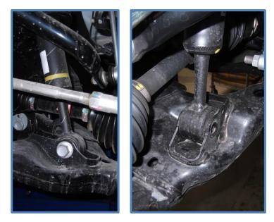
10. Remove the three nuts from the upper mount and remove shock.
