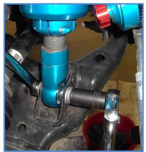
18. Connect the upper control arms using the instructions provided with your UCA kit. Now is a good time to check clearance with the UCA and shock installed, cycle the UCA past the fittings and make sure the UCA does not make contact with hose or fittings. It may be necessary to adjust hose and fittings depending on your set up.
