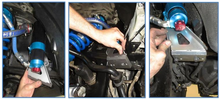
25. Bolt the sway bar to the bottom of the reservoir bracket using the supplied 3/8 X 3/4" bolts (CB4702). Tighten bolts to 35 ft-lbs. Repeat steps 20-23 on opposite side of vehicle. Reinstall skid plate after both sides are done.
