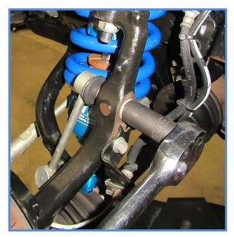
27. Tighten reservoir clamp with a 3/16 Allen wrench using the supplied 1/4 X 1" SHCS (CB1501)
