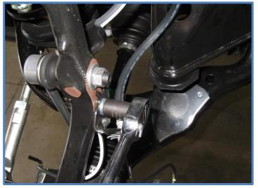
6. Disconnect sway bar link by removing the nut using a 17mm wrench or socket. If the sway bar link stud is spinning you may need to hold the stud with a 6mm Allen wrench.
