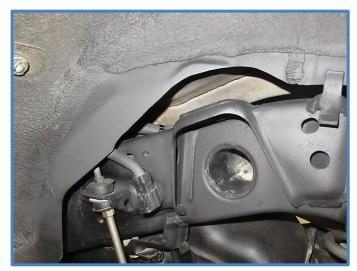
• You must also remove the factory bump stop and replace with a factory style 4Runner or FJ Cruiser bump stop. Failure to modify the bump stop will reduce available wheel travel and cause the rear axle to bottom out prematurely on the factory bump stops that were designed to work with the air bags.
