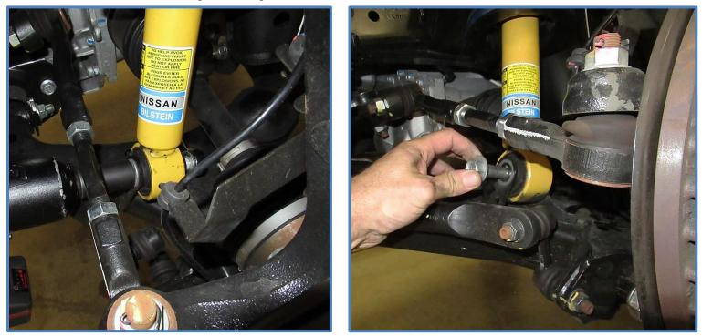
3. Disconnect tie rod – Remove the cotter pin, then remove the nut using a 22mm wrench or socket. Separate the tie rod from the knuckle.
