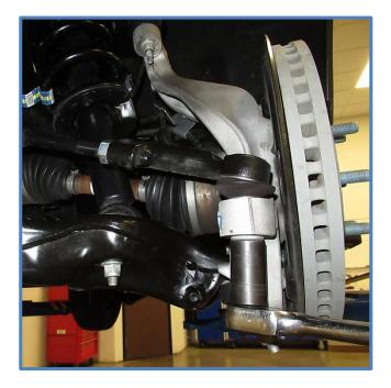
4. Remove the nut from the sway bar link using an 18mm socket.
