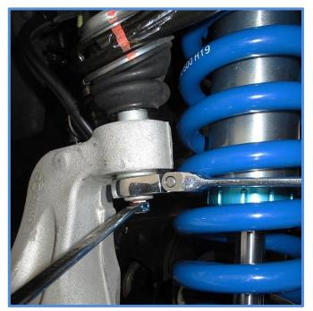
13. Reconnect the tie rod and torque to factory specs.
