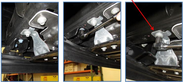
Place the reservoir mount against frame between the frame and tow hook (and skid plate if applicable). Install the two tow hook factory bolts you just removed. If you have the skid plate option you will need to place one of the thick washers from the hardware kit (CW1701) between the frame and skid plate, install factory bolt and tighten. Tighten all bolts to factory specs. Reservoir brackets are side specific, see photos for proper mounting.
