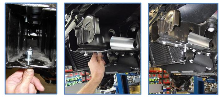
9. Install King Remote Reservoir Shocks by first feeding the reservoir through the hole at the top of the shock mount, then place the shock in position on the vehicle. Get the shocks in position on both sides of the vehicle before reconnecting any suspension components. Shocks are side specific, the reservoir will route towards the front of vehicle as shown below.
