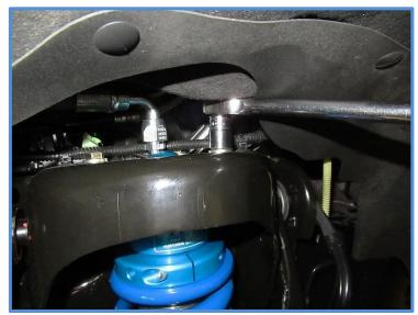
11. Line up the lower mount and use the supplied 12mm bolts and washers along with the factory nuts. Torque the lower shock bolts to 75ft/lbs. using an 18mm & 19mm wrench/socket.
