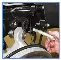
5. Remove the 3 nuts from the upper mount of the shock using a 15mm wrench/socket and remove the shock.
