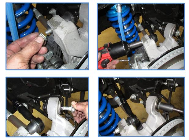
9. Reconnect the sway bar links and tighten to factory specs.
