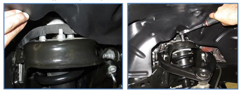
3. Disconnect the upper control arm. Remove the nut using a 21mm socket and separate a-arm from knuckle.
