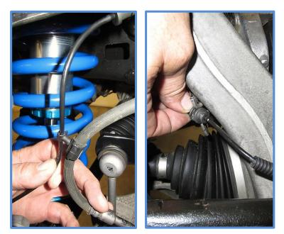
16. Place the reservoir in the reservoir bracket. Use the provided hose clamps to secure reservoir to the bracket.
