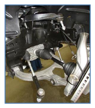
7. While the shock is removed, bend the ABS clip towards the knuckle about a 1/4" or so. You will check clearance when the shock is installed.
