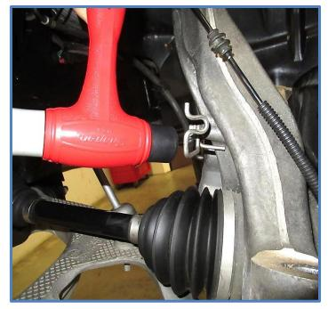
8. <u>Installing King Shocks</u> – Be aware the shocks are side specific, make sure you are installing the shocks on the correct side. Begin placing the shock in position on the vehicle while feeding the reservoir between the upper control arm and the upper mount "coil bucket".
