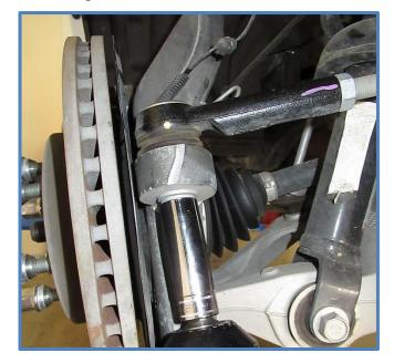
5. Remove the lower mounting bolt using a 21mm wrench or socket on the bolt head and a 24mm wrench or socket on the nut. Remove the nut then pull the bolt out.
