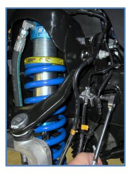
15. <u>Install Reservoir Brackets and Reservoirs</u> – First remove the two bolts from the frame above the skid plate using a 13mm socket. Then remove the bolt to the rear of the skid plate using a 15mm socket. Do one side at a time!
