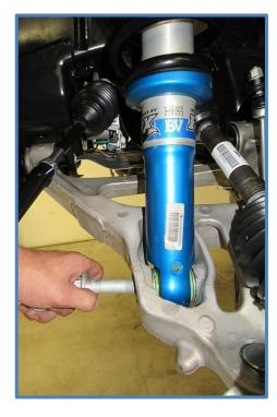
5. Remove the upper ball joint nut using an 18mm socket. Separate the upper control arm from the spindle.
