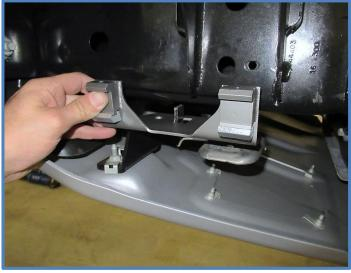
17. Push the skid plate back into position against the frame. Replace and tighten the two factory bolts you just removed. Then replace and tighten the rear skid plate bolt. Repeat steps 15-17 on opposite side of the vehicle.
