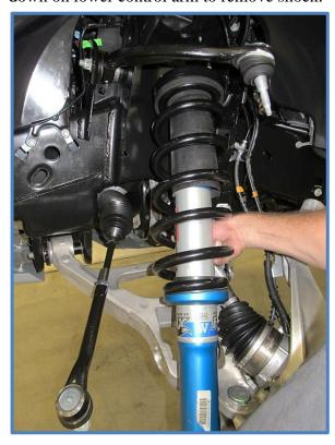
8. <u>Install King Shocks</u> – Place the coilover in position on the vehicle by inserting the upper mount with mounting studs into the upper mount (coil bucket) on the vehicle. Then, while pushing down on lower control arm, get the rod end into the mounting pocket on the lower control arm. Be aware the shocks are side specific and can only be mounted on the designated side. Photos below show the left side.
