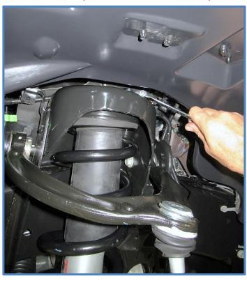
7. Remove factory shocks. You will need to push down on lower control arm to remove shock.
