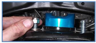
10. Install factory lower mounting bolt and nut but do not tighten yet.
