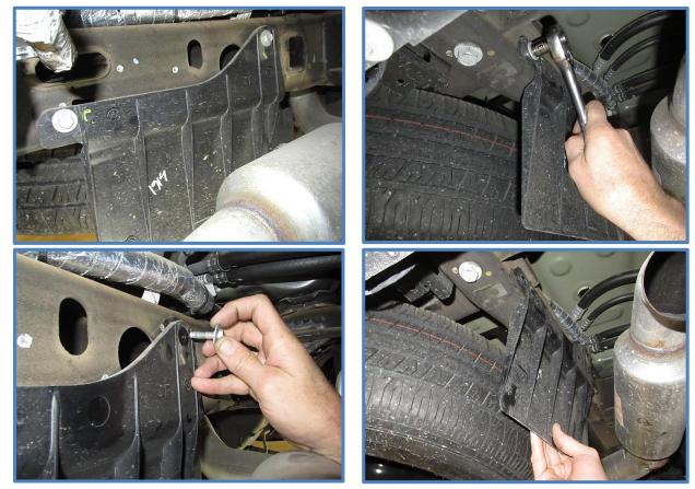
11. Place the reservoir bracket on the frame lining up the holes in bracket with the two holes in the frame where you just removed the plastic guard. Place the plastic guard over the reservoir bracket, reinstall the factory bolts and tighten to factory specs.
