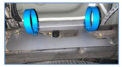
15. Install Reservoirs – Slide reservoir into clamps as shown.
