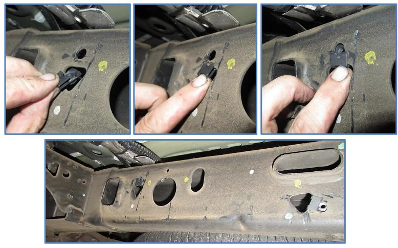
13. Attach reservoir bracket to the nut plates in the frame using the provided 1/4" bolts and washers...
