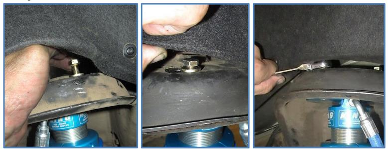
7. Install the lower mounting bolt and tighten to factory specs.
