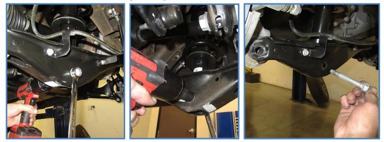
3. Remove the upper mounting nuts using an 18mm wrench/socket.
